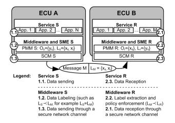
Figure 2: Overview of the framework architecture. A labeled message M is exchanged between 2 applications (App.) of S and R services through a secure channel. L and O designate the service label and ownership.  $x_s$ ,  $y_s$  and  $x_i$  are secrecy/integrity tags.
